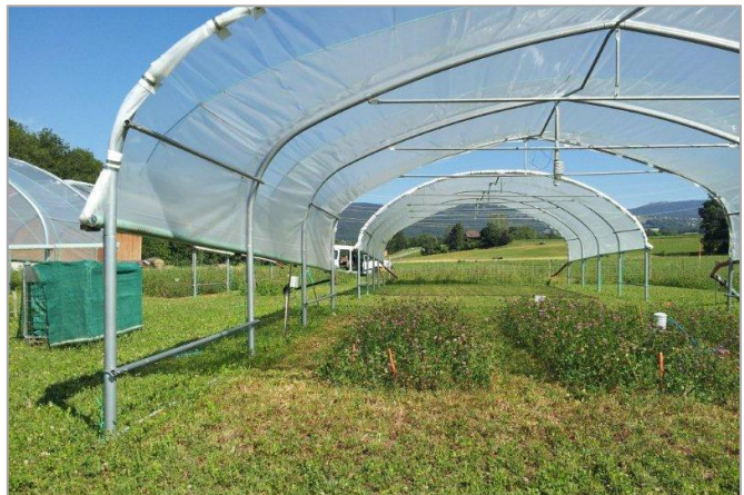
Droughts are simulated with the help of growing tunnels.
