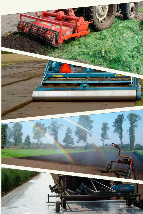
Fig. 1: Anaerobic Soil Disinfestation in a glance (from top to bottom): Incorporation fresh organic matter Closing the surface Wetting the soil Covering with virtually impermeable film (VIF)
