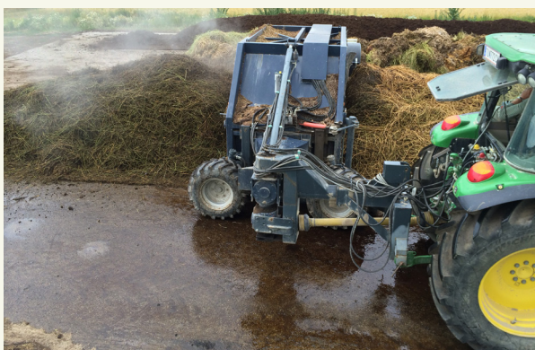
Fig. 1: Homogenizing resources for thermophilic compost production with a compost turner
