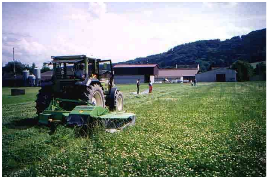
Fig. 3. Tractor with mower fixed at the side, mowing the white clover field
