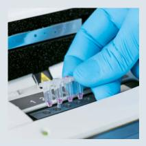
releasing the DNA. Two control test-tubes, each containing one specimen of the quarantine organism in question, also form part of the testing kit. The four tubes are inserted in a detection device that is smaller than a shoe box. There, the sample is heated to 65 degrees Celsius. At this temperature, a DNA polymerase makes copies of specific sections of the genome.
