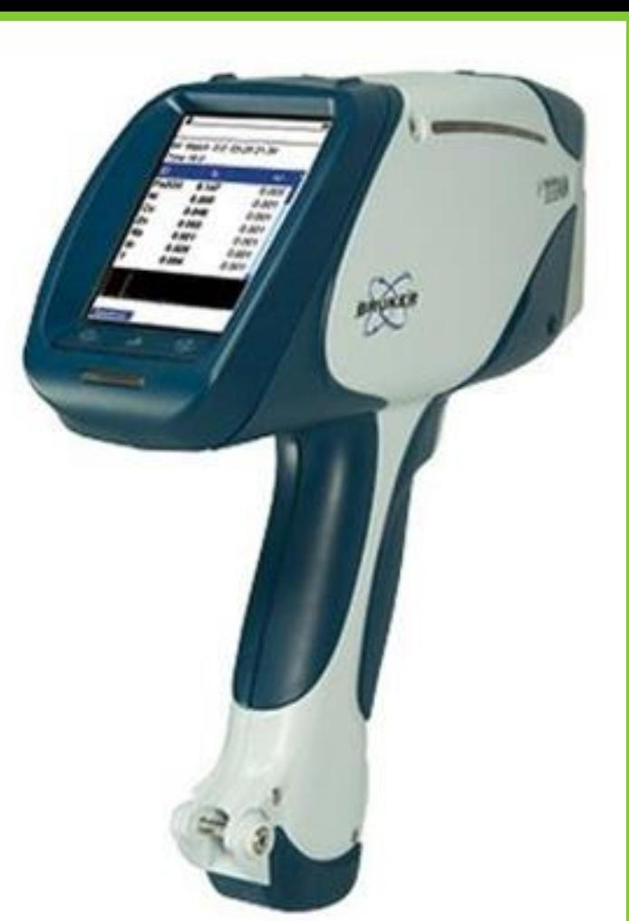
To compare the relative elemental concentration between the organs, the XRF data are carefully corrected with a **calibration test**. In this example, the % of S determined by a isotopic ratio mass spectrometer (IRMS) is correlated with the value of %S measured by XRF Titan. The equation relying % S from IRMS and XRF is applied directly in the instrumental software.
