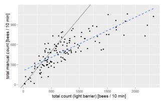
**Figure 3** Data from a trial in April 2020. Total ("in+out") count from the light barriers compared to manual counts at the hive entry, scaled to correspond to 10 minutes of accumulated data. To guide the eye, the black line is the y=x diagonal, while the blue, dashed line is a simple linear fit to the data.
