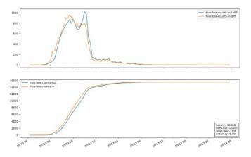
**Figure 4** Robbers test for one counter, the count is from the light barrier at the food source. The upper panel shows the bee count per 10 minutes for incoming bees (orange) and leaving bees (blue). The lower panel shows the aggregated counts.
