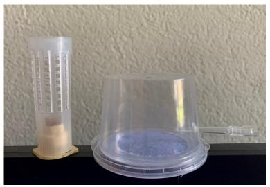
Figure 4 Left: Assembled Nicot cage with feeder cup, right: clear bell plast cage with pipet tip feeder
