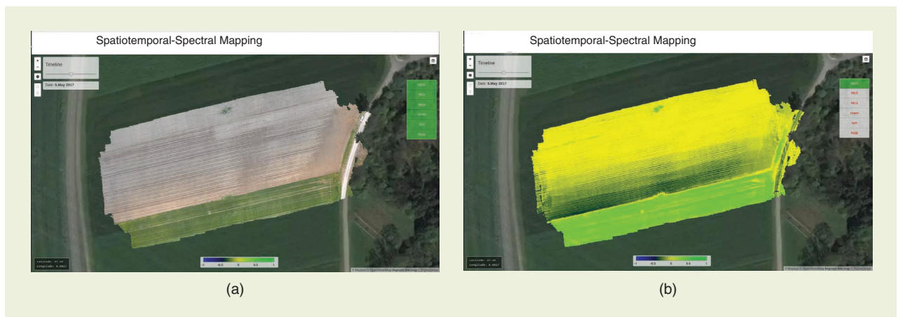
Figure 9. A visualization interface for the spatiotemporal spectral database showing (a) RGB orthomosaics and (b) the corresponding index maps for a sugar beet field over time. The user can select spectral layers to view a georeferenced reflectance orthomosaic corresponding to a wavelength band, view the color orthomosaic, and toggle through all of the available surveys using the timeline. (Images courtesy of Flourish.)
