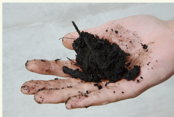
Fig. 3: Fist test: Compost has the right moisture content.
