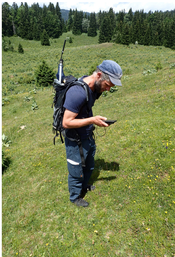
Fig. 9 | Mapper with smartphone operating the ALL-EMA app. The GPS receiver is carried in his backpack.
