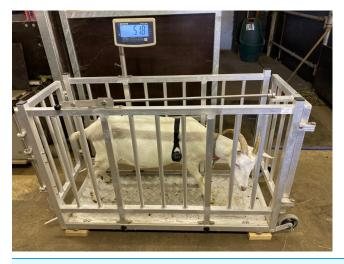
Figure 2 Picture of a dairy goat standing on the scale and wearing the harness used to record cardiac<br/>measures.Full-size 🖬 DOI: 10.7717/peerj.12893/fig-2
