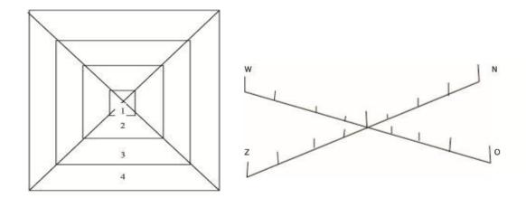
**FIGURE 4.5.** DESIGN OF THE X PLOT (AFTER GB COUNTRYSIDE SURVEY HANDBOOK 2007). THE LENGTH OF THE SIDES ARE INSQUARE 1: 2.00M, 2: 5.00M, 3: 7.07M AND 4: 10M. THIS PRODUCES NESTED PLOTS OF RESPECTIVELY 4  $m^2$ , 25  $m^2$ , 50  $m^2$  AND 100  $m^2$ .
