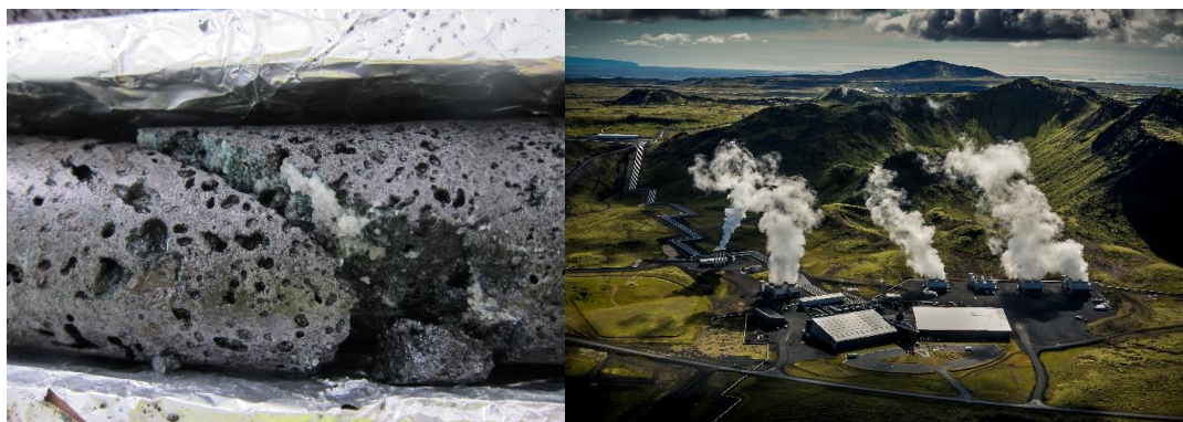
Figure 14. Left: a bore core with mineralized atmospheric CO 2 from the world's first DACS plant at the Hellisheidi geothermal powerplant (right). 77
