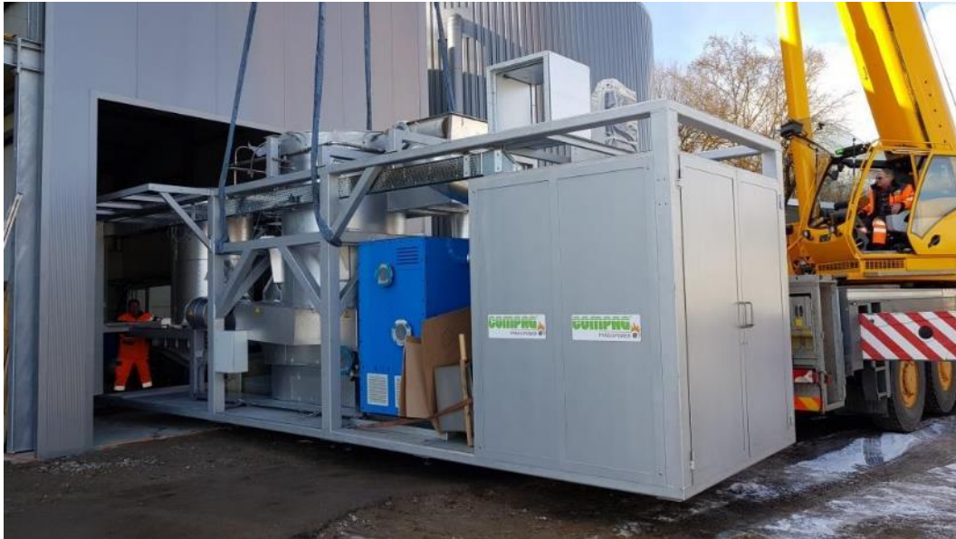
Figure 10. COMPAG CPP800 unit for 2'400 t/a wet or dry wood chips and wood screening residues. The unit produces 50 kW electric power with a hot air turbine and up to 350 kW heat for greenhouse heating. The expected biochar production is to 400 t/a. Picture taken during delivering of the first unit to a bigger organic farm with greenhouses in Region Zürich, January 2019.
