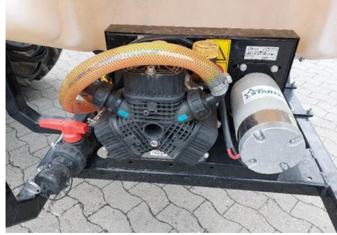
Measured at a pressure of 5 bar = 38 l/min
