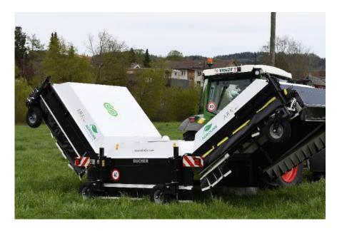
3 independent units equiped with cameras, 6 m working width
