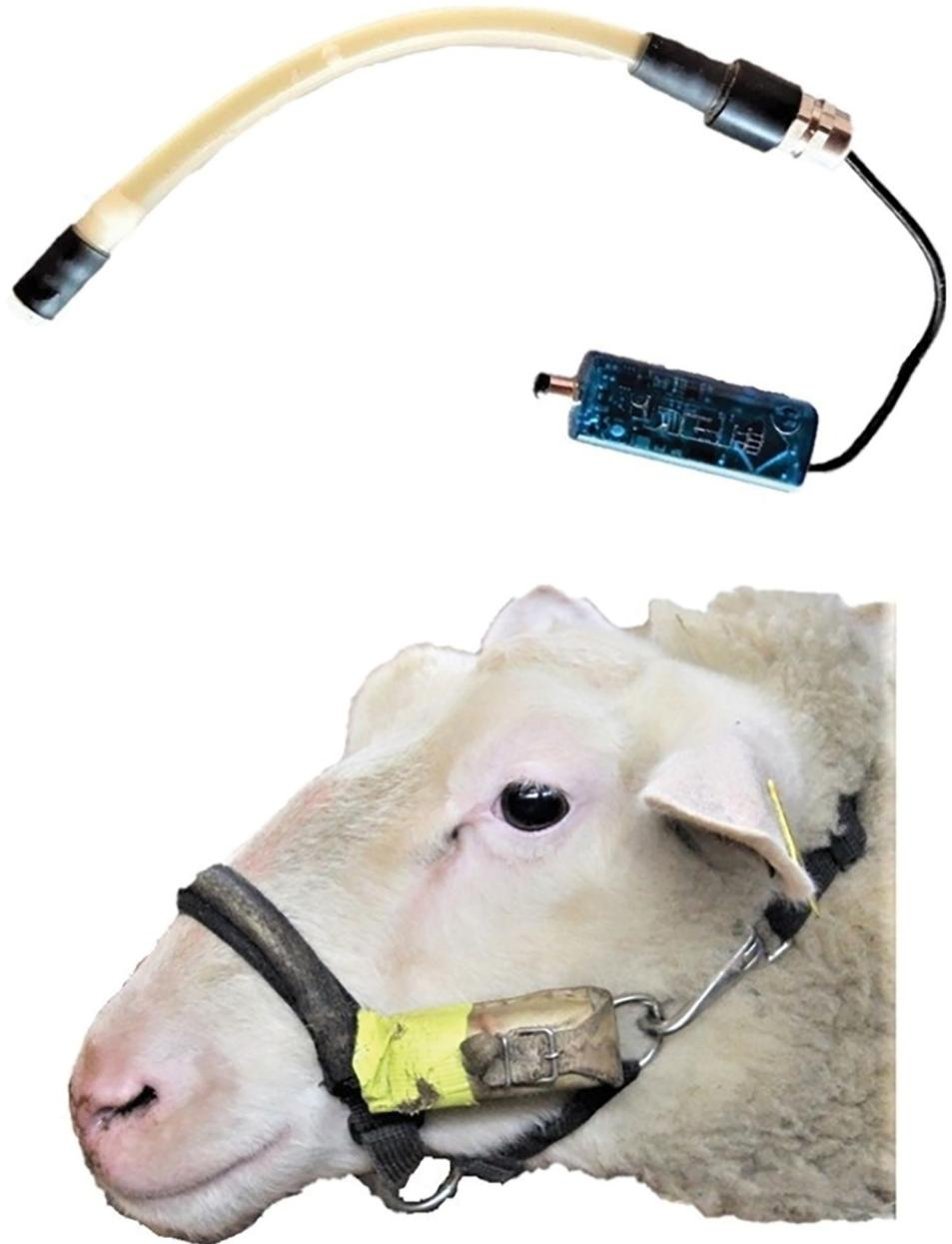
**Fig 1. MSR-jaw-movement recording system outside the halter (top) and integrated in the halter worn by a sheep (bottom).**
