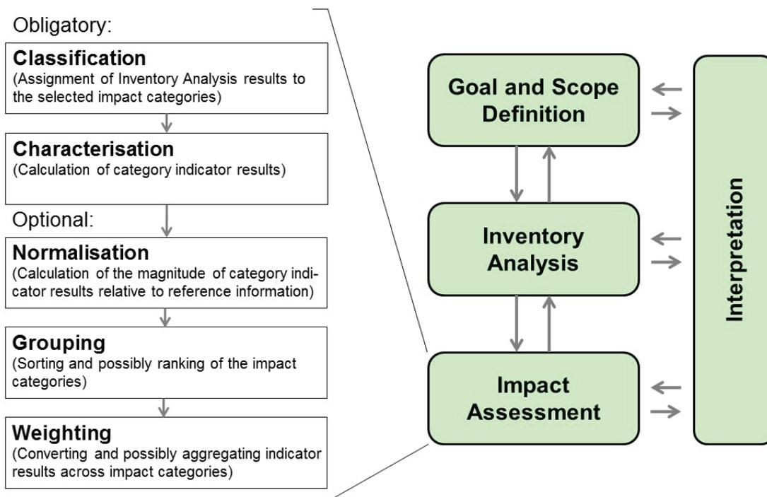
Figure 5.2: Life-Cycle Assessment (LCA) framework according to ISO Standards 14040 and 14044.
