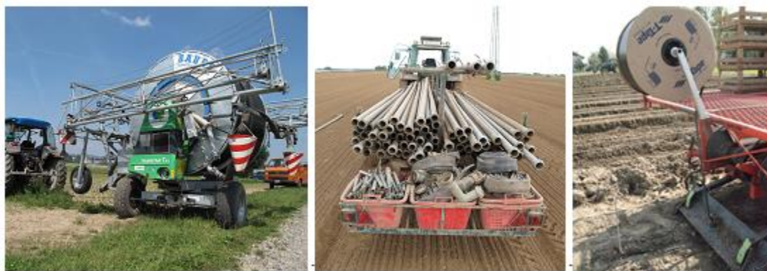
Figure 2. Left: mobile sprinkler (Rollomat), center: assembly of fixed sprinkler, right: laying of drip irrigation (source: ART).
