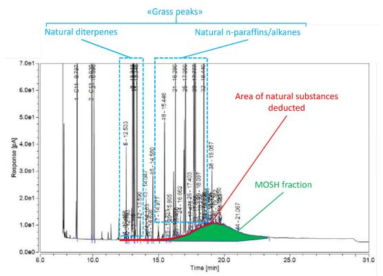
Figure 1: Analysis of a MOSH chromatogram using the example of a butter sample
