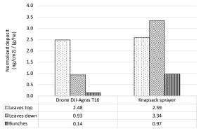
Figure 2: Quantification of product deposition in the different compartments of the foliar hedge using a fluorescent marker in Paudex (VD) in 2020. Comparison of the deposit obtained during the last treatment in August with the DJI AGRAS T16 drone and a backpack sprayer.
