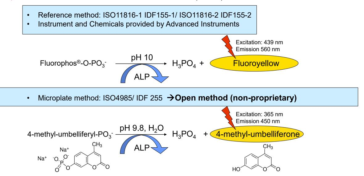
Based on: Ziobro G.C., McElroy K.M., Fluorometric Detection of Active Alkaline Phosphatase and Gamma-Glutamyl Transferase in Fluid Dairy Products from Multiple Species. Journal of food protection. 2013, 76(5), pp. 892–898
