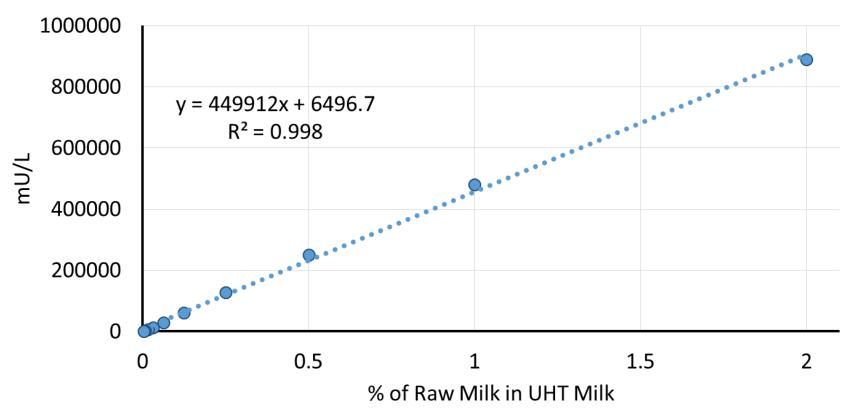
Detection of 0.003 % of Raw Milk in UHT Milk possible  $\rightarrow$  similar as Reference method Calculated limit of detection: 15 mU/L
