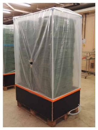
Figure 1 | Automated experimental unit manufactured by Agroscope, which allowed potatoes to be treated independently in the same cold room. (Photo: Margot Visse-Mansiaux, Agroscope)
