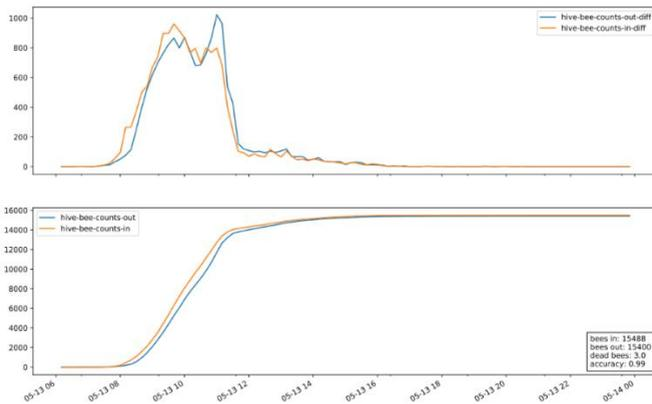
**Figure 4** Robbers test for one counter, the count is from the light barrier at the food source. The upper panel shows the bee count per 10 minutes for incoming bees (orange) and leaving bees (blue). The lower panel shows the aggregated counts.
