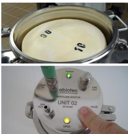
Fig. 1: Dynamic gas volume measuring system developed in collaboration with abiotec Ltd., Rheinfelden, Switzerland
