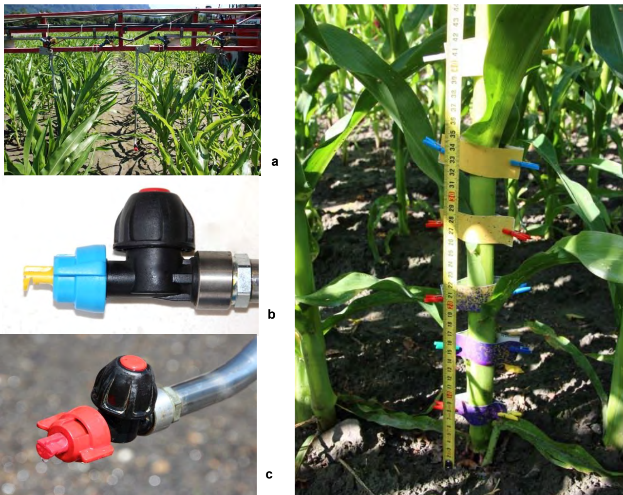
Fig. 24: Use of droplegs at an advanced growth stage of maize (a). The spray droplets are only deposited on the lowest part of the shoots whereas the leaves remain unsprayed (picture at the right). For that purpose the dropleg carries a 140 degree deflector nozzle which points towards the ground (b, c). The chosen height of the nozzles on the droplegs above the ground (height of the boom above ground) determines the width of the spray swath on the ground.
