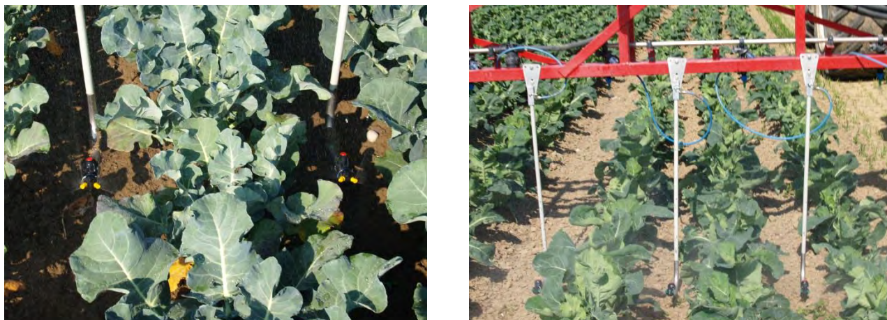
Fig. 13: Droplegs with each two deflector nozzles combined with flat fan injector nozzles on the boom in broccoli and cauliflower.
