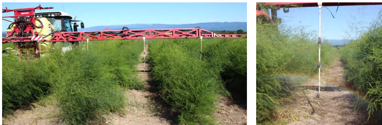
Fig. 22: Preliminary spray trial in asparagus on the 18 th of July 2012 with a special version of droplegs with a length of 120 cm and with three pairs of deflector nozzles caliber 05; row distance 1.8 m, spray broth volume 1000 l/ha at a pressure of 5 bar and a forward speed of 5 km/h.
