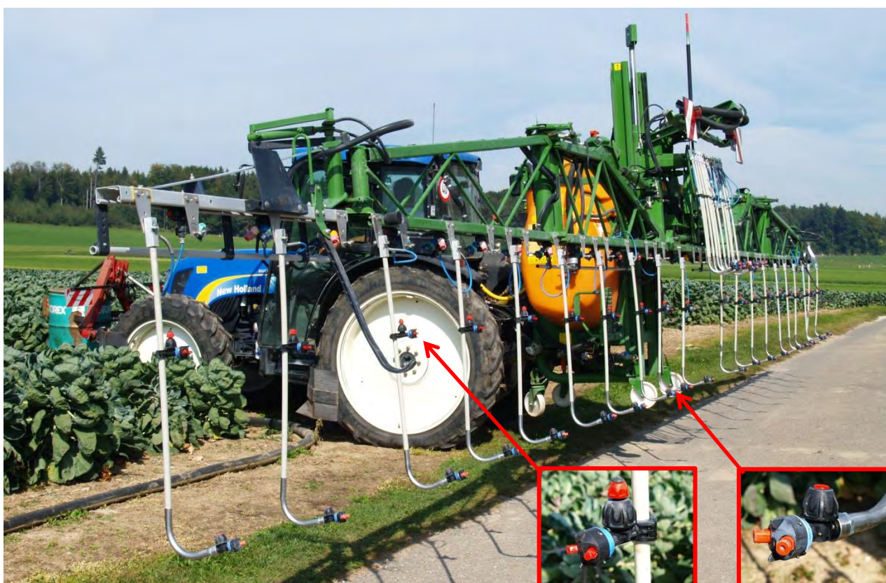
Fig. 1: Droplegs with each two pairs of deflector nozzles for the application of fungicides and insecticides in Brussels sprouts. The top nozzles on the boom remain closed.
