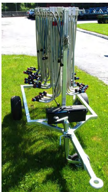
Fig. 28: Examples of racks built by growers for quick and easy storage of droplegs.
