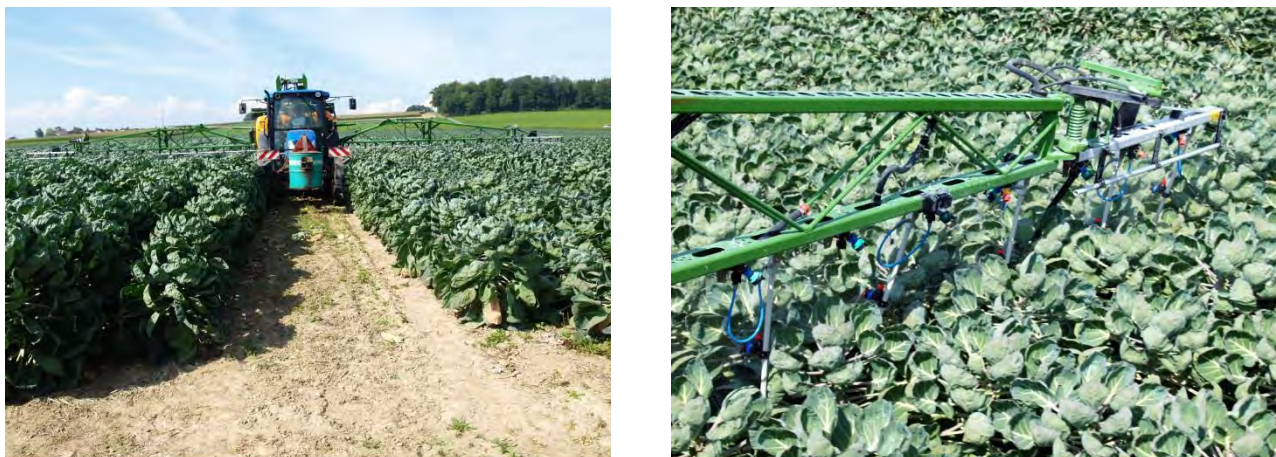
Fig. 12: A special version of the dropleg with two pairs of nozzles at a low and upper level (see also fig.1 and 6) is particularly useful in tall crops such as Brussels sprouts. At early crop stages the top nozzles on the dropleg are shut down. The dropleg is carried through the crop with all four nozzles travelling within the canopy thus drift due to wind is reduced very much.
