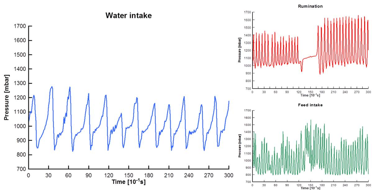
FIGURE 2: Comparison of pressure profiles during water intake, rumination and feed intake, taken from the same animal and noseband sensor, plotted over 30 seconds
