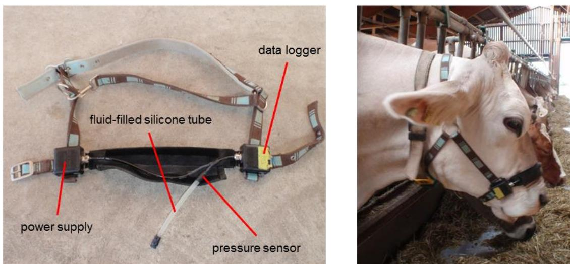
FIGURE 1: RumiWatch noseband sensor containing a fluid-filled silicone tube with built-in pressure sensor and two electronic units
