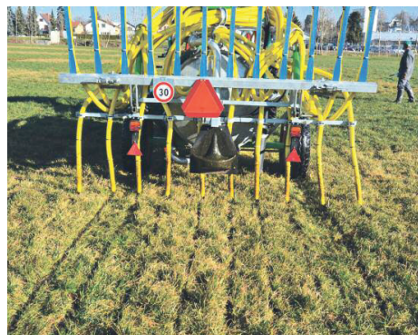
Tuyaux (pendillards) souples.
