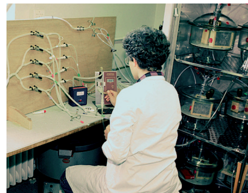
Trial setup for screening essential oils and there components under laboratory conditions against Varroa destructor .
