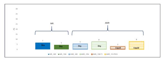
Fig. 2 – Mean relative repeatability for each method tested in a range of concentration 140 000 -1 100 000 cells/mL
