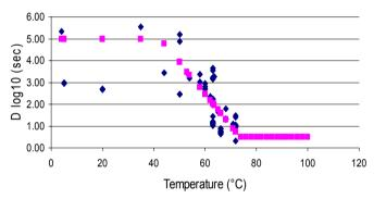
Figure 1: D values as a function of the heating temperature of milk. Values <50°C are lower limits or estimates of D in anaerobic environments. Within the interval of 54-74°C, a linear regression is seen (red spots). The 5 (T<40°C) and 0.5 (T>75°C) horizontal spots represent estimates of D. In both temperature intervals, the behaviour of D is not temperature dependant. Neither cooling nor completely kill MAP.
