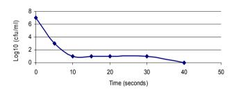
Figure 2: MAP survival during milk pasteurisation at  $63^{\circ}$ C. The D value only describes the 10 first seconds of pasteurisation (killing). The overwhelming part of time, MAP shows different temperature dependent behaviour (survival; afssa Report of the 5<sup>th</sup> Workshop, Paris, 24-25 of October, 2002).
