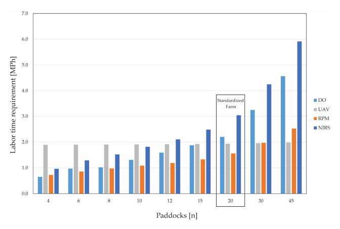
**Figure 3.** Labor time requirement of three smart farming tools and direct observation (DO) in measuring herbage mass (and quality) on a model farm with a 28.8 ha milking platform and different paddock numbers. UAV, unmanned aerial vehicle; RPM, rising plate meter; NIRS, near-infrared reflectance spectrometer analysis with cutting samples.
