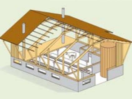
The Modular Construction Standards for Farm Building Costs is a tool for planning low-cost buildings.
